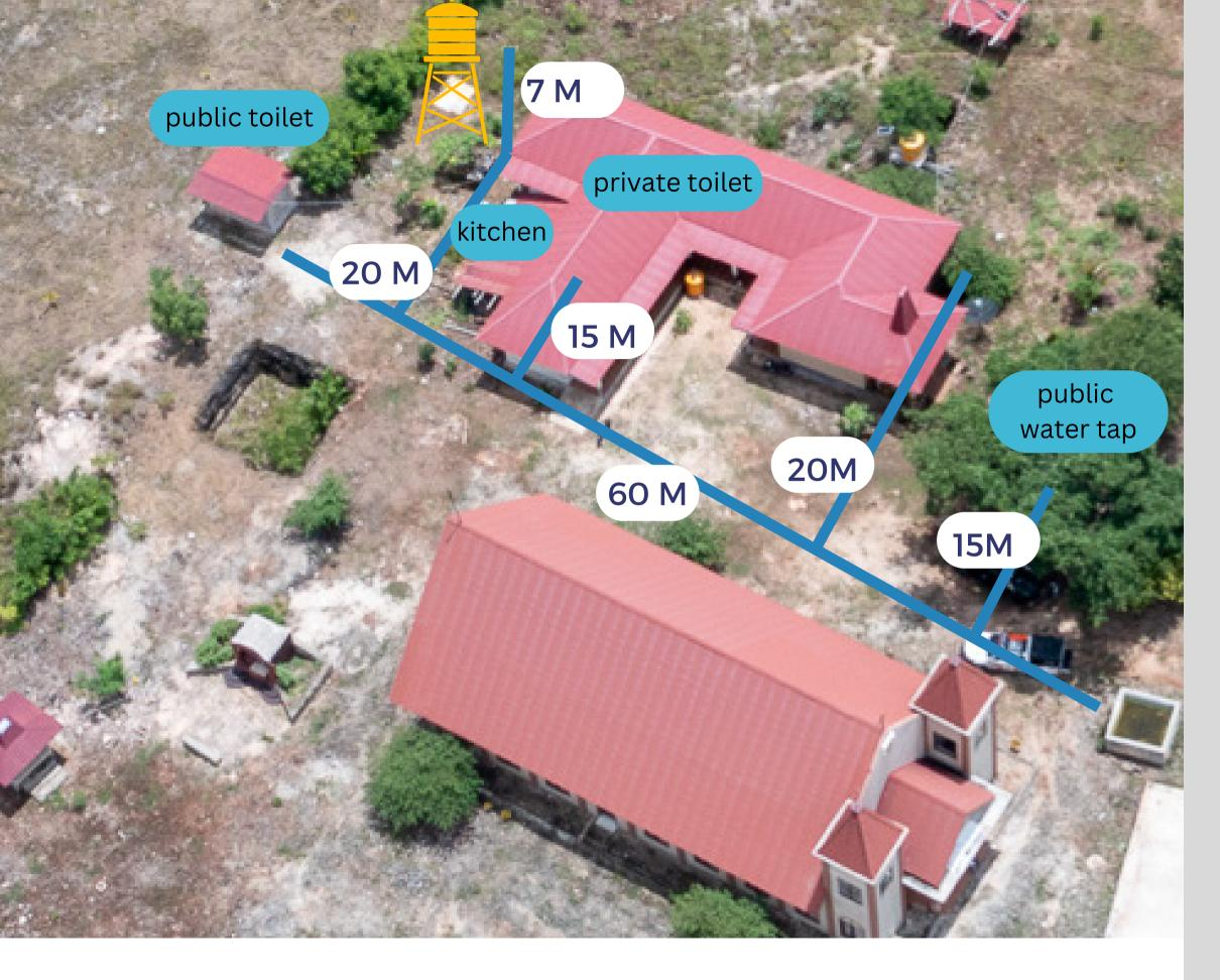
SUBMERSIBLE PUMP 0.5 HP AUTOMATIC PRESSURE PUMP KABEL, STOP KONTAK, BOX CONTROL PIPA HDPE 1" 150 METER + CONNECTOR PIPA (PVC 1" & 1//2") 30 METER + KNEE L, T
